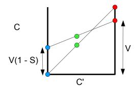
The example shows a base colour of orange. Its red component,  $C'_R = 1$  and this has been reduced to C = V. At the same time, the blue component  $C'_B = 0$  has been increased to C = V(1 - S). The green component has been moved to lie on the new line as well. Now you can see why when V = 0, the colour is black regardless of the hue. You can also see why, when S = 1, both ends of the line are at the same height – V, so the colour is grey.
