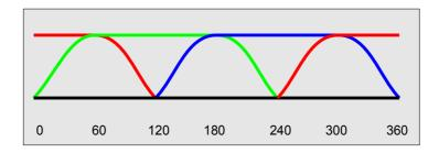
Systems which use **hue** as one of their components are called 'cylindrical' or 'conical' systems because one of their components is an angle, not a value. In a computer, the angle is still represented as a number between 0 and 255, however.
