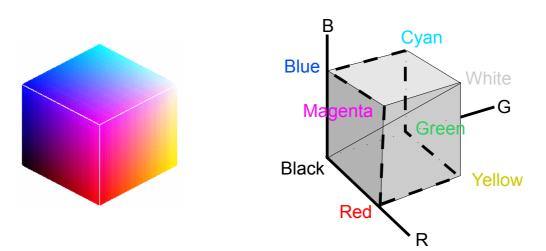
It will be noted that black and white are at the ends of the principal diagonal of the cube while the three primary colours and the three secondary colours (known as **principal** colours) lie on a wiggly line which threads through all the remaining six corners.
