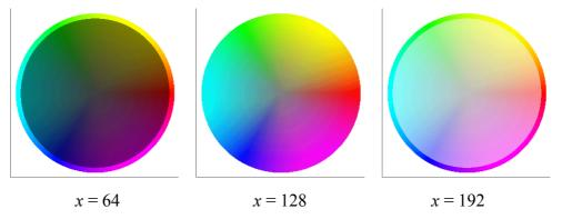
This system is sometimes called the bi-conical system because from x = 0 to x = 128, the colours expand from the black corner of the colour cube; then in the second half they contract down to pure white.
