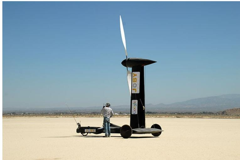
The turbine is coupled to the wheels by a drive chain.
