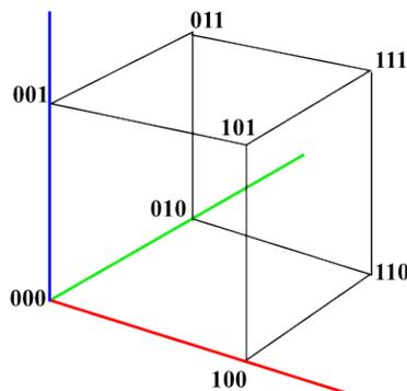
Fig 2: Configuration space of a 3-colour LED
