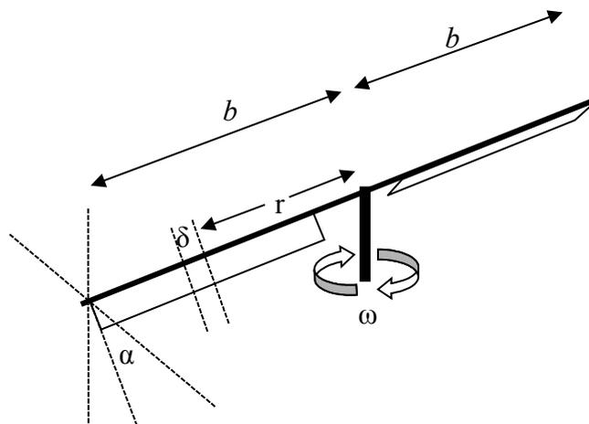
To calculate the lift produced we must integrate along the length of the blade. Consider a small element of the blade at a distance  $r$  from the axis and of length  $\delta r$ . Its horizontal velocity through the
