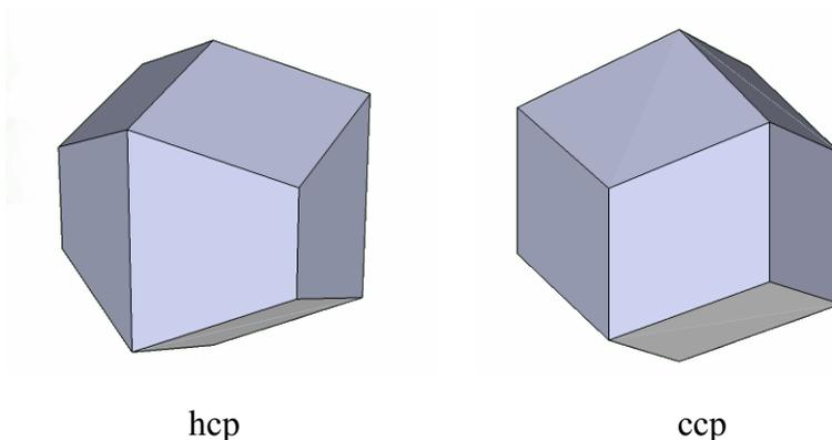
Both solids have 12 quadrilateral faces but in the case of the Wigner-Seitz cell for the cubic close-packed lattice, all the faces are identical rhombuses with the smaller angle being equal to  $70.53^\circ$ . This solid is a rhombic dodecahedron. It is immediately obvious that the ccp lattice has a much higher degree of symmetry than the hcp lattice.
