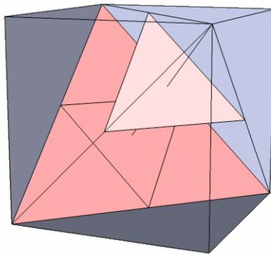
Now since the spheres in the triangular planes are in contact, it is clear that the diagonal of the cube has length 2 sphere diameters. The size of the unit cube for the face-centred lattice is therefore  $\sqrt{2}$  diameters in length.
